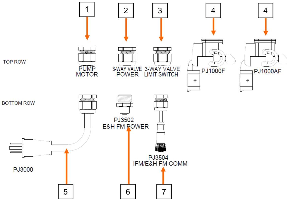
1. Cable from pump motor connects to this connector . Prewired at the manufacturing plant.
