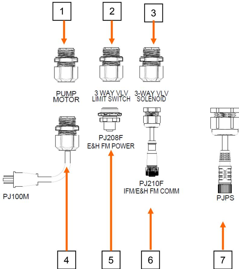
1. This terminal is for the pump motor power. Prewired at the manufacturing plant.
