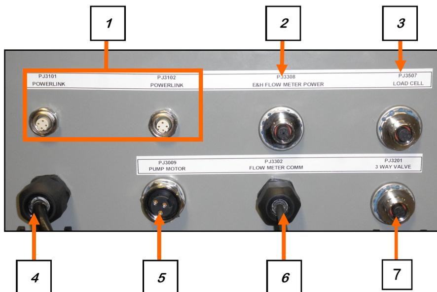
1. Connect a cable with four pin connector to one of the two Powerlink connectors. Connect the other end to the Powerlink connector on the closest control panel. Repeat this process until all control panels are connected. It may be Treater to Tri-Flo® to Bin Site panel etc. The order or number of devices is not important. It is important that all panel are connected. All pump stand control panels will need to be connected in a similar configuration.
