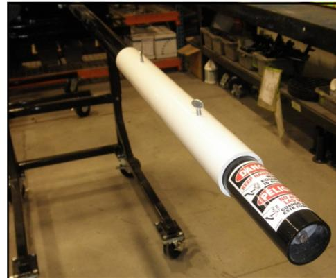
*Calibration Sleeve at end of Auger Tube*
