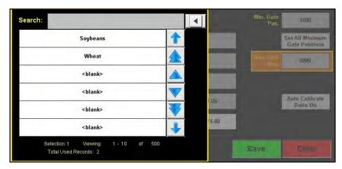
**1A. MINIMUM GATE POSITION:** Pressing this button brings up a keypad to enter a value for a minimum gate position for this individual seed profile.
