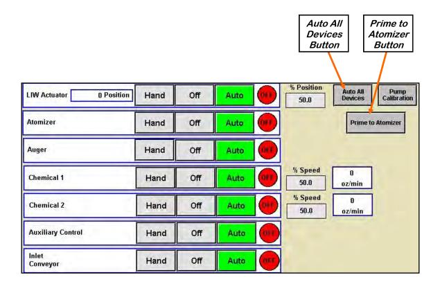
3. Return to the main screen and press the Start Setup button. Press the gray buttons to change the Recipe or Seed Type fields. Press Start to begin the run. The atomizer and auger will turn on. Open the manual gate on the box. When the proximity switch detects seed, a timer will count down the number of seconds the start delay was set for. When that time elapses, the slide gate will open.
