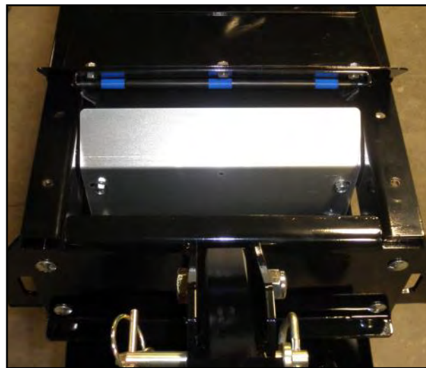
Bottom clean-out cover removed
