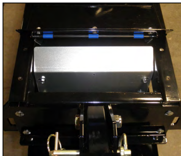
Bottom clean-out cover removed
