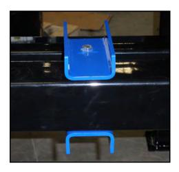
**STEP B:** Remove all four of the shipping support brackets. Save for reuse if treater is moved.
