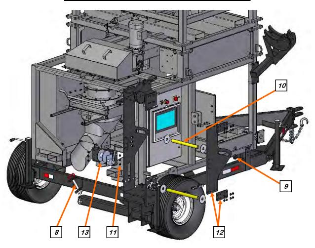
14. Using a forklift and choke strap, find the approximate center of the auger assembly and lift it. You may have to set it back down and lift several time to find the correct balance point. With a second person guiding one end of the auger from the ground, slowly move the auger so it is parallel to the right side of the treater. Raise it until it is slightly higher than the cradle. Slowly move it forward until it is lined up with the cradle.
