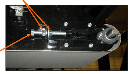
Use this bolt to tighten and align the belt
