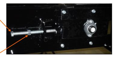
Tighten jam nut after adjustment
