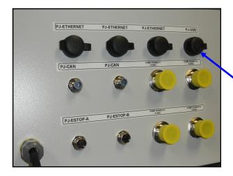
The USB port located on the bottom of the Main Control Panel allows the operator to download reports to a compact flash device.
