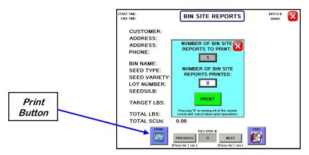
4. If the Auto Print Bin Site Report has been activated on the Print Set-up screen (see page 40) steps 2 and 3 will not be required. The print verification screen will appear and automatically print the number of reports specified.
