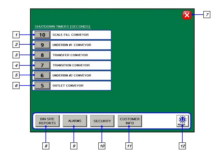
NOTICE When buttons 1-6 are pressed, a numeric touch pad (right) will appear allowing the operator to enter in a number for that particular parameter.
