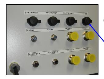
There is a USB port located on the bottom of the Main Control Panel that can be used to download reports to a compact flash device. The flash device must be in FAT 32 format.
