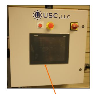
HMI screen on LPX Manual Control Panel
