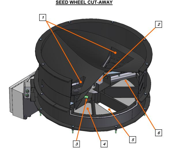
1. Openings to Wheel: This is where the seed is dispensed into the wheel pockets.
