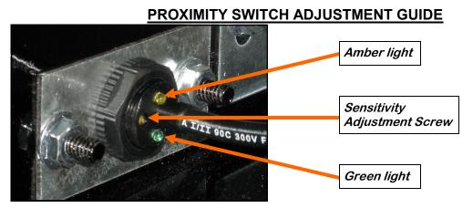
The proximity switches mounted in the extension ring and the seed wheel detect when seed is present.
