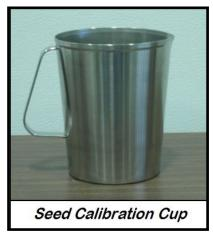
5. After the cup has been filled, strike off the top of the calibration cup with a straight edge (see page 31, figure 2).
