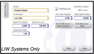
the operator to the Seed Editing screen. You must press the Save button again to confirm the updated calibration ratio.
