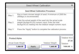
Pressing Seed Calibration causes a pop up screen to appear that allows for the calibration of the seed variety for the Seed Wheel.
