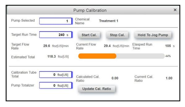
5. Repeat the process as necessary and for each different chemical slurry used.
