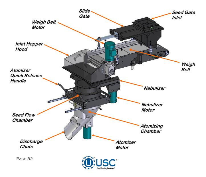
The Illustration below shows how seed passes through the nebulizer and atomizing chamber. The red represents treatment being dispensed to the seed as it passes through the chamber. After the seed passes through the atomizer, it goes into the drum where the coating process is completed.
