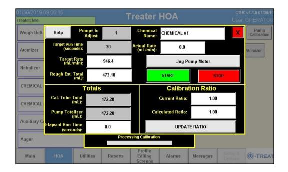
Repeat this process for each pump The ration could be slightly different due to hose wear.
