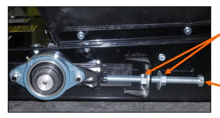
Loosen the jam nuts before adjusting the bearing position bolt
