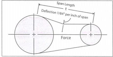
MEASURE THE SPAN LENGTH "T" AS SHOWN IN THE SKETCH ABOVE.
