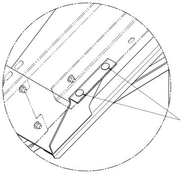
LOWER STOP MOUNTS IN THE LAST 2 HOLES OF LOWER ANGLE, FROM HEAD END. NOTE DIRECTION OF STOP.
