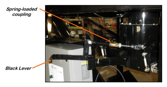
When the black lever is pushed up, the seed gate is in the <u>open</u> position, and seed will flow through.
