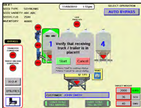
The system displays the current weight of seed in the weigh hopper.
