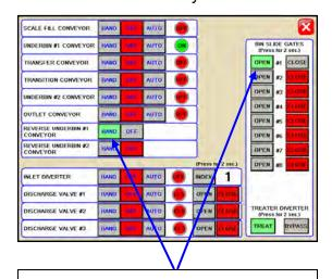
Press the "HAND" button and then place the bin slide gate to the "OPEN" position.
