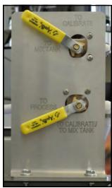
Place the MIX TANK / CALIBRATION TUBE valve that is located on top of the pump stand to the calibration tube position.
