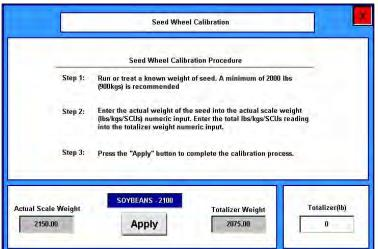
Note: The seed wheel calibration screen will adjust the seed profiles Cups / Pocket Ratio automatically.
