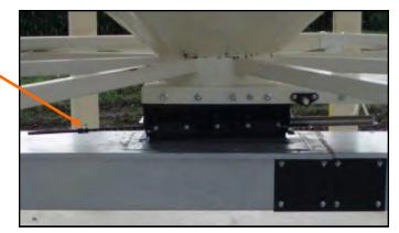
3. Finally, set the position of the manual slide gate that is located under the weigh hopper. This gate will control the flow of seed out of the weigh hopper by restricting the size of the opening from the weigh hopper. The more open the gate is, the faster seed will exit the weigh hopper. To set this gate, simply loosen the three nuts on the gate. Then adjust the gate to the desired position, and retighten the nuts.
