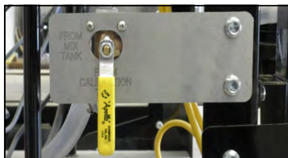
Drawing chemical from the bottom of the Calibration Tube
