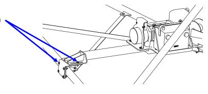
8. Remove the lever stop bracket from the winch assembly. This allows access to the clutch release lever on the winch. Rotate the lever to allow the spool to free wheel. Pull the cable out of the winch for routing through the pulleys.
