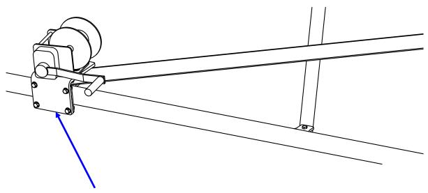
5. Remove the limit switch assembly and set aside. Loosen the six 3/8 bolts and slide the mounting plates out to the end of the adjustment slots.
