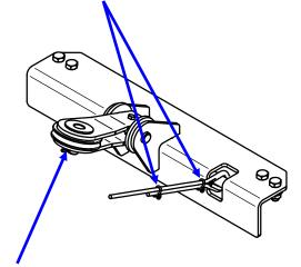
3. Remove cotter pin, pulley pin and the pulley from the upper cross member. Set aside for re-installation later.
