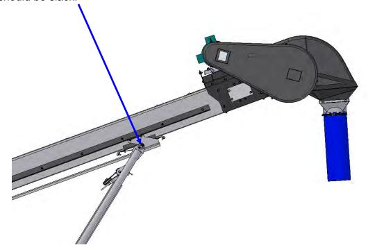
2. Once the cable is slack, remove cable clamps and cable from anchor.
