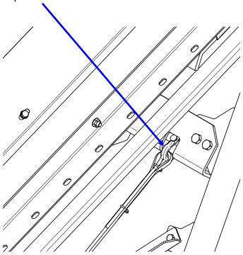
11. Rotate clutch release lever back into operating position. Re-install the lever stop bracket and tighten hardware.
