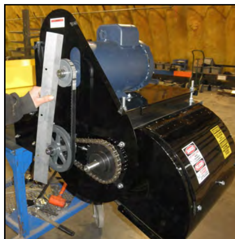
Lay a straightedge across pulley faces
