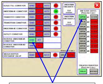
Press the HAND button and then place the bin slide gate to the OPEN position.
