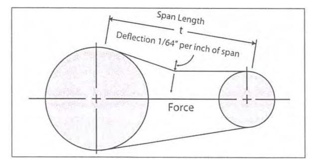
The following range of deflection forces are normally adequate for a used drive belt.
