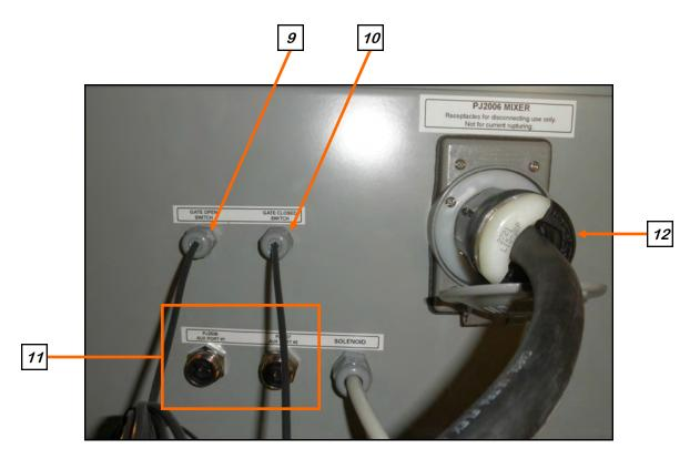
Use the diagram located above the pneumatic control assembly to make the connections from the ports on the bottom of the assembly to their respective locations.
