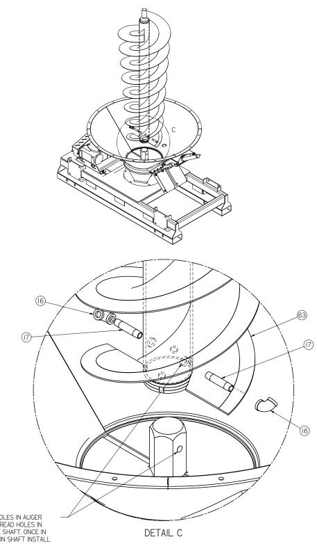
ALIGN HOLES IN AUGER WITH THREAD HOLES IN IN DRIVE SHAFT. ONCE IN PLACE ON SHAFT INSTALL FITTINGS AND SET ANGLE OF ELBOW AROUND 30 DEGREES ABOVE HORIZONAL.
