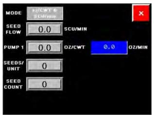
MODE: oz / CWT & SCU / min - User will need to enter the seed information in the Seeds / Unit and Seed Count blocks as well as enter the treater seed flow in SCU / min and oz / CWT to calculate the oz / min (shown in blue on right side of screen) to be applied.
