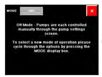
MODE: Off - Allows the user to control the pump through the pump setting screen
