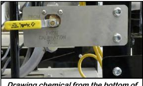
Drawing chemical from the bottom of the Mix Tank
