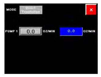
MODE: Direct Translation – Allow user to set pump to oz / min. The rate the user enters will be the rate at which the pump will operate.
