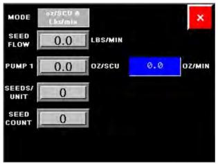
MODE: oz / SCU & Lbs / min - User will need to enter the seed information in the Seeds / Unit and Seed Count blocks as well as enter the treater seed flow in Lbs / min and oz / SCU for the pump and it will calculate the oz / MIN (shown in blue on right side of screen) to be applied.
