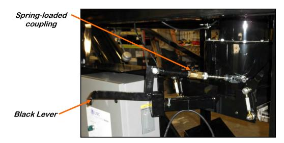
When the black lever is pushed up, the seed gate is in the <u>open</u> position, and seed will flow through.
