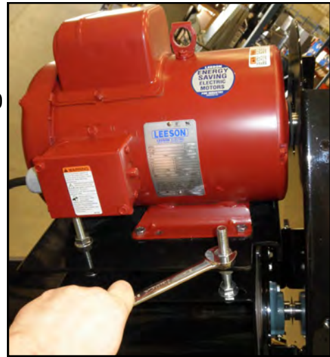
Motor base adjustment
