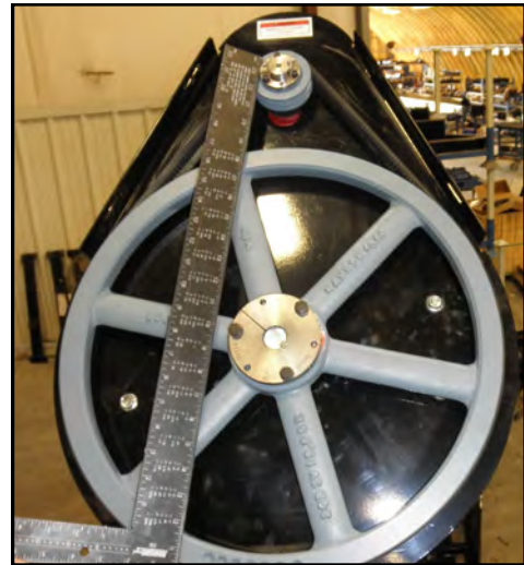
Lay a straightedge across pulley faces
