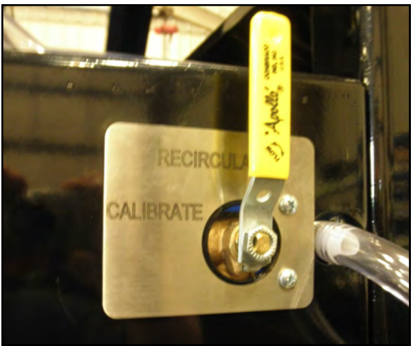
Directs Liquid back into the top of the 5 gallon tank
