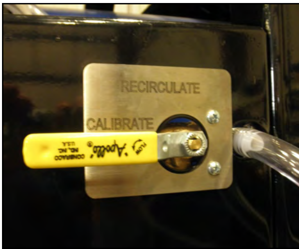
Directs liquid to the hose to the right of the valve to check calibration
