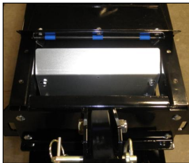
Bottom clean-out cover removed
