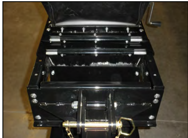
Bottom clean-out cover removed
