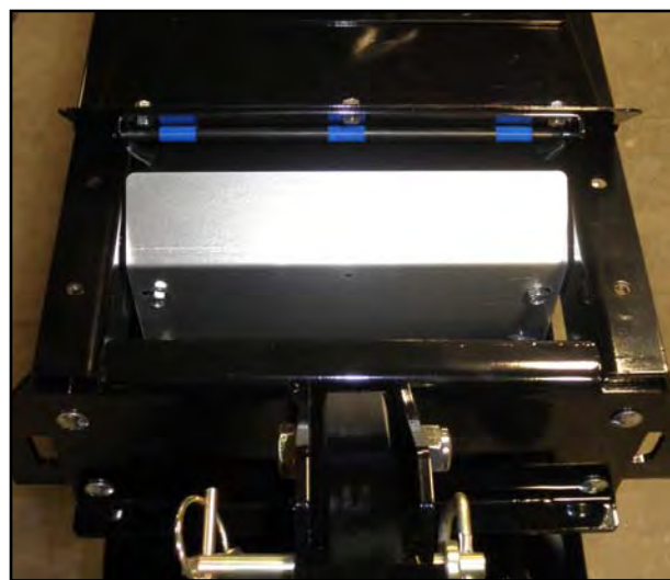
Bottom clean-out cover removed
