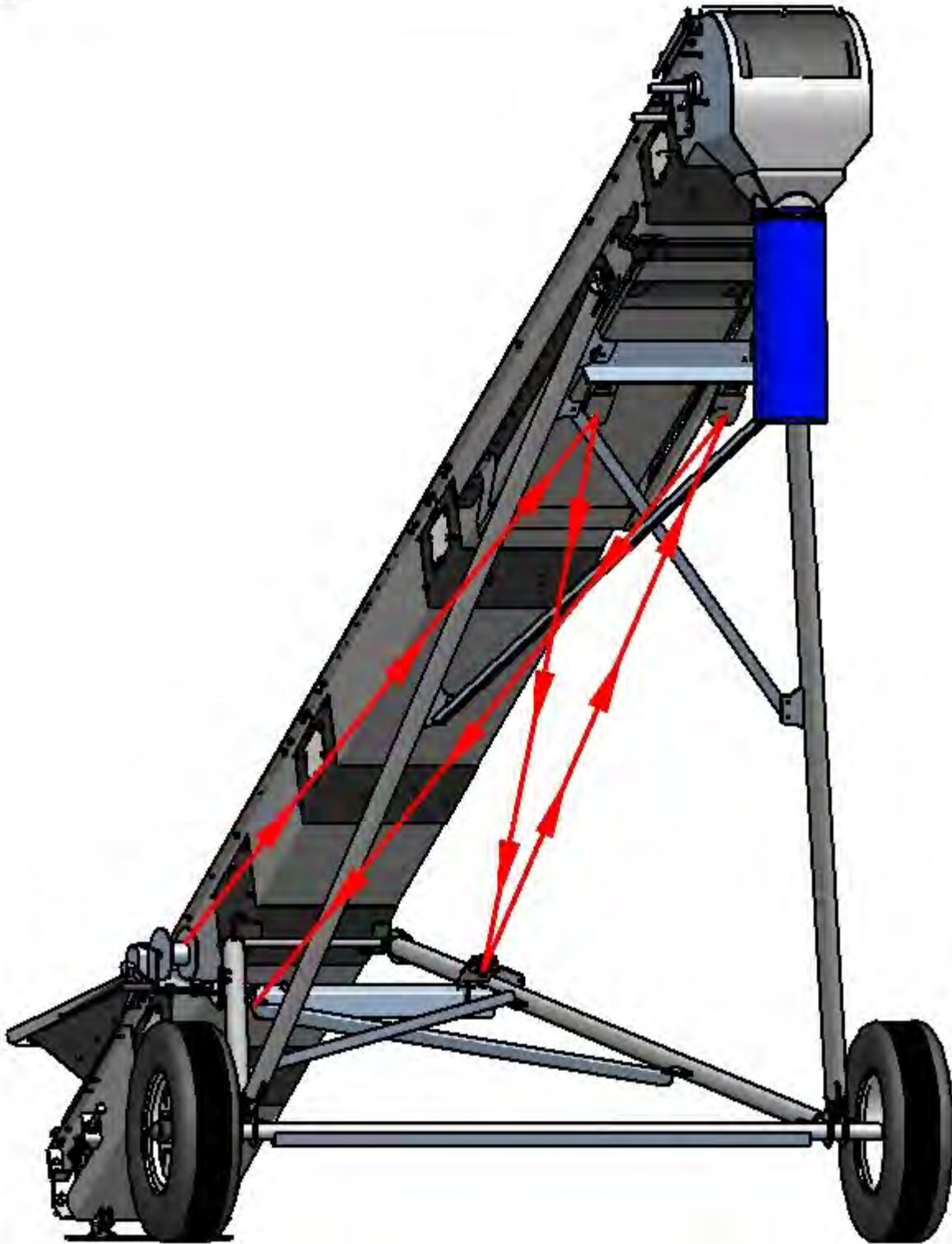
TYPICAL CABLE ROUTING
