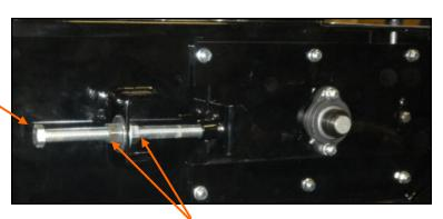
Loosen these jam nuts before adjusting the bearing position bolt
