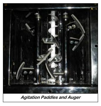
The dry product is dispensed through small openings in the auger tube to create a curtain affect when the dry products are applied. The tube may be rotated to increase or decrease the coverage area.
