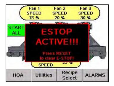
During an Emergency Stop, the ESTOP ACTIVE will be displayed on the screen and the system will be halted. To continue, the operator will need to pull all ESTOPS out and then press the RESET button on the front of the panel.
