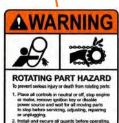
3. Do not operate with rotating parts exposed.
