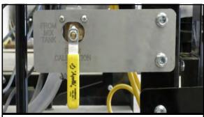
Drawing chemical from the bottom of the Calibration Tube
