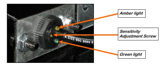
The proximity switches mounted in the extension ring and the seed wheel detect when seed is present.
