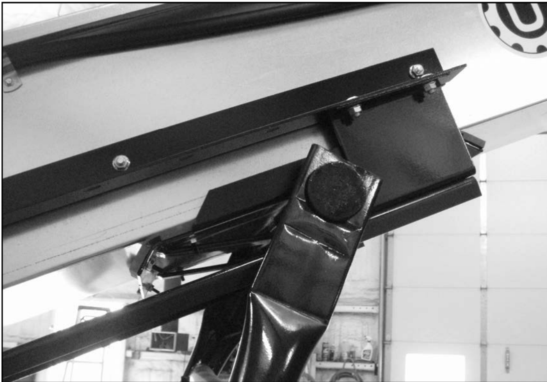
Picture of Slide Assembly after Installation
