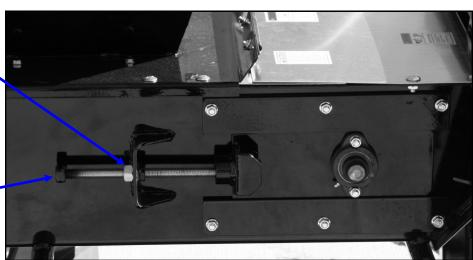
Use this bolt to tighten and align the belt
