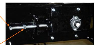
Tighten jam nut after adjustment
