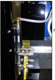
7. For LPX, LX and MX treaters, attach the chemical tubing from the pump stand(s) to the atomizer plumbing on the seed treater (left). For all other treaters additional tubing can be added or removed to accommodate your set-up.
