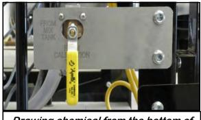
Drawing chemical from the bottom of the Calibration Tube
