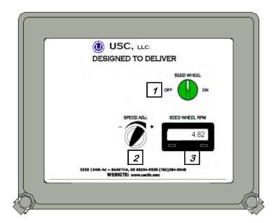
1. Seed Wheel: Allows the operator to turns the seed wheel on or off.
