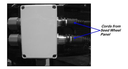
3. Wire the Inlet Conveyor Proximity Switch into the small junction box located on the seed wheel. The Blue wire on the proximity switch will connect to the terminal opposite of the Red wire with Black stripe. Two other Blue wires will also be connected into this terminal. The Black wire on the proximity switch will connect opposite of the White wire with Black stripe.
