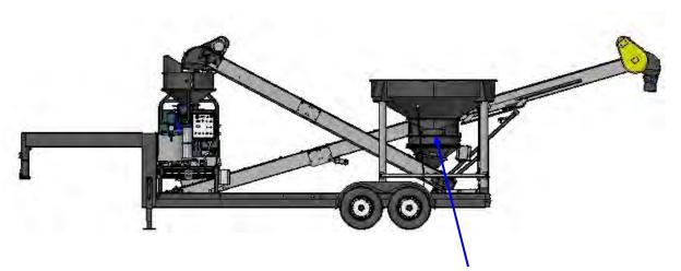
Seed Wheel under hopper on Portable Seed Treater.
