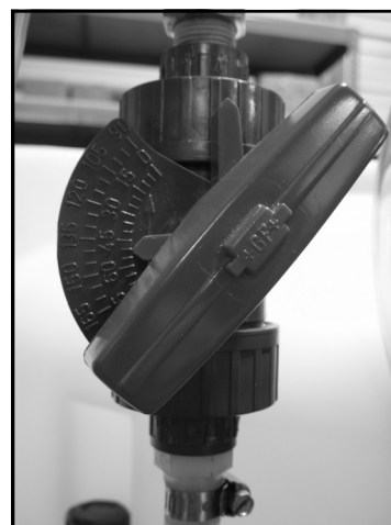
Metering Valve at Dial Setting 50
