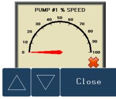
*<u>7. Screen "EXIT" Button</u>*: This button is used to exit back to the previous screen. Its functionality is the same throughout the HMI display.
