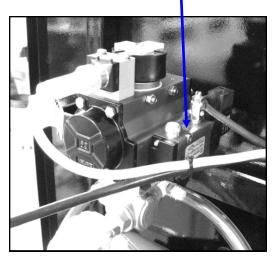
12. Connect a dedicated analog phone line to the modem located in the top left portion of the control panel. This will allow USC remote access to the seed treater to help diagnose and fix problems that may arise.
