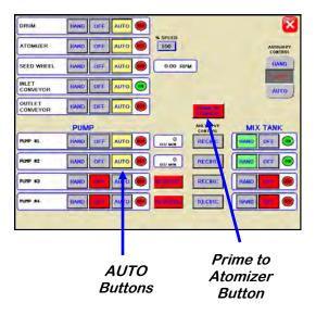
3. Advance back to the main screen and press the "STARTUP" button. The drum, atomizer, inlet conveyor and outlet conveyor will activate. The pump will turn on and re-circulate until it reaches the desired flow rate needed to match the target treating rate that was entered. Begin the flow of seed into the inlet conveyor. The inlet conveyor will then begin dumping seed into the seed wheel.
