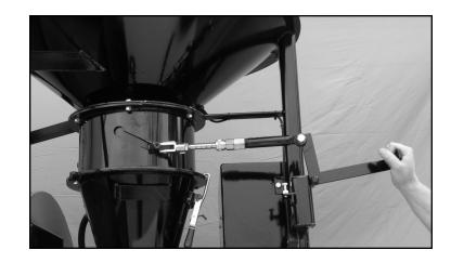
When the black lever is pushed up, the seed gate is in the <u>open</u> position, and seed will flow through
