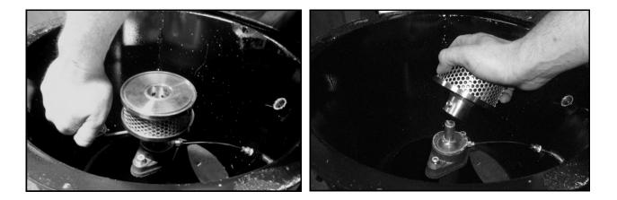
4. The atomizer head is threaded together. Unscrew the head for better access to cleaning.
