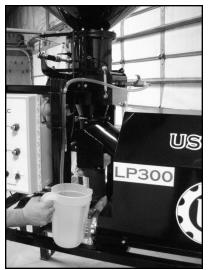
Calibrating pump with measuring cup.
