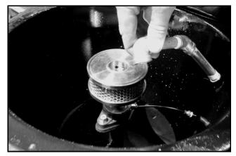
3. Use a 3/16" allen wrench and loosen the set screw located on the bottom of the atomizer head. Next remove the head from the shaft.
