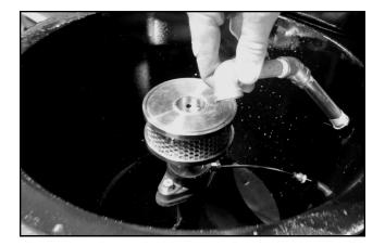
3. Use a 3/16" allen wrench and loosen the set screw located on the bottom of the atomizer head. Next remove the head from the shaft.
