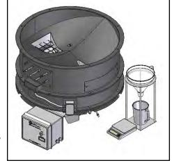
The purpose of the seed wheel is to simplify calibration and make seed flow calibration more accurate. The seed wheel saves time when switching to different seed sizes and seed types, and can be mounted to most LP800 and LP2000 models.
