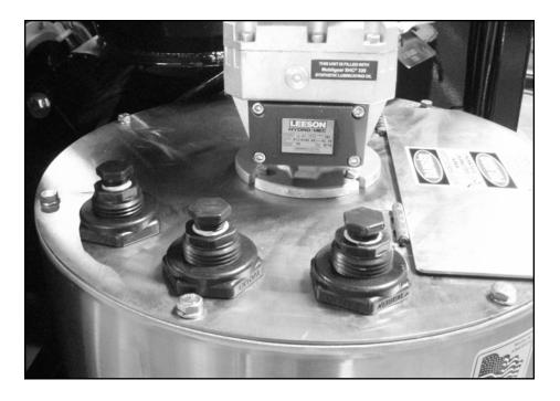
Pump #1 liquid system is also equipped with a calibration tube, which is used to determine the liquid flow rate. The calibration tube measures in ounces on a 0-340 scale. Three-way valves direct liquid from different areas to keep all liquid contained.
