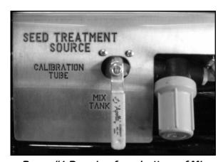
Pump #1 Drawing from bottom of Mix
